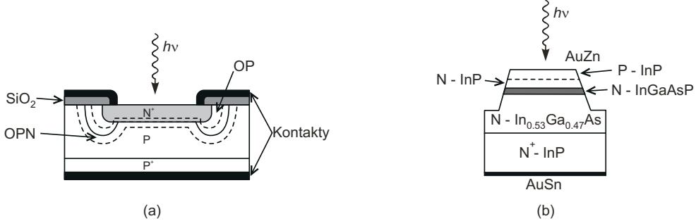
Obr. 23: Lavinová fotodioda (APD) a) Si APD b) InGaAs/InP APD
