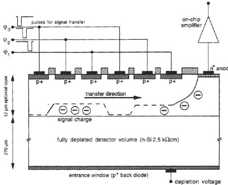
Obr. 34: CCD element.
