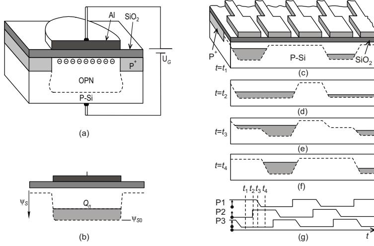
Obr. 33: CCD element.
