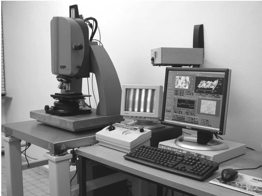
Figure 5.3: Zygo NewView 5000 noncontact 3D surface profiler.
